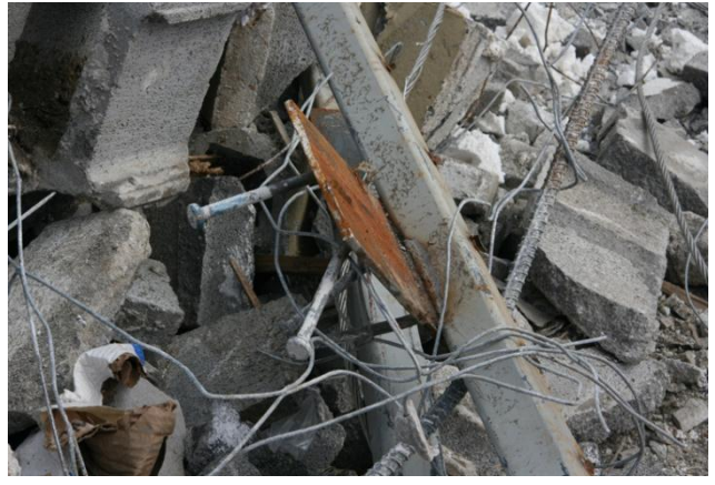
Photo 27: Embed plate with short studs pulled free from top of CMU wall.
