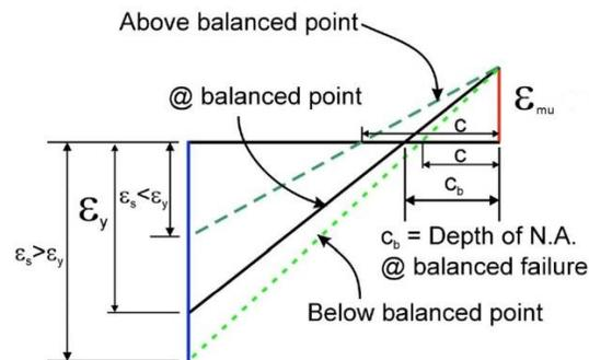
Figure 4: Critical Strains used to Evaluate Points on an Interaction Diagram
