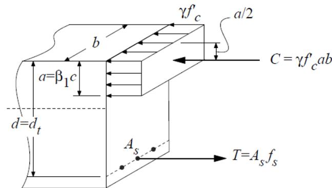
Figure 3: Equivalent Stress Block
