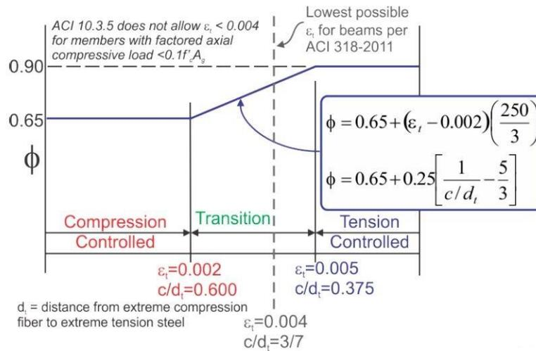
Figure 2: Strength Reduction Factors for Reinforced Concrete in Compression and Flexure
