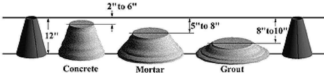
Figure 1: Typical Slumps for Concrete, Mortar, and Grout
